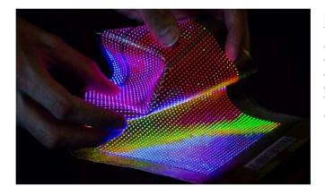
Researchers from Holst Centre (set up by TNO and imec), imec and CMST, imec's associated lab at Ghent University, have demonstrated the world's first stretchable and conformable thin-film transistor (TFT) driven LED display laminated into textiles. This paves the way to wearable displays in clothing providing users with feedback.
